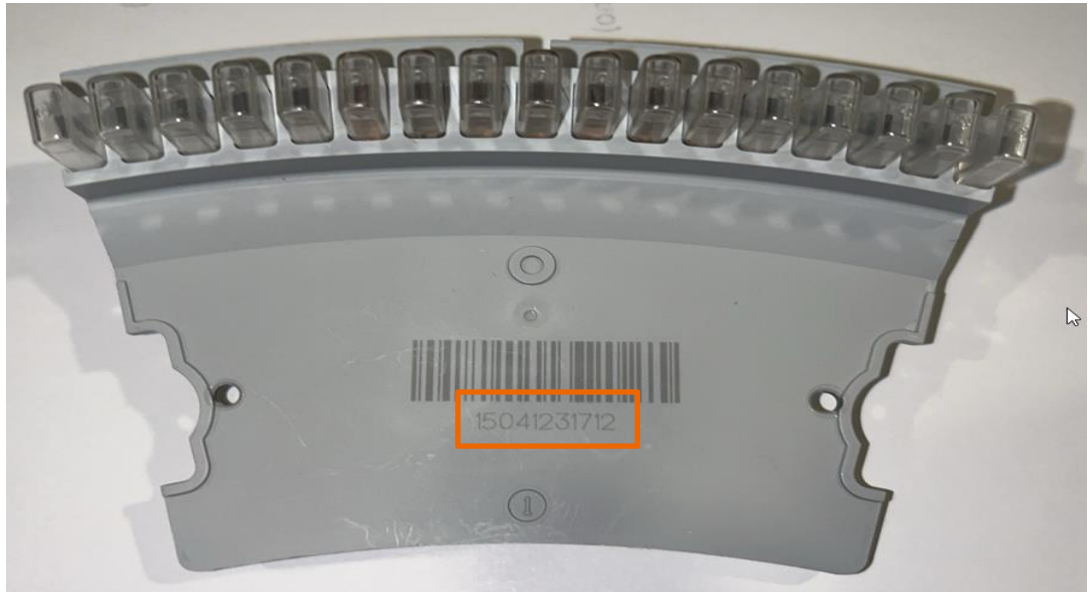
Figure 1. Location of the lot number on Atellica CH Reaction Ring Cuvette Segment
