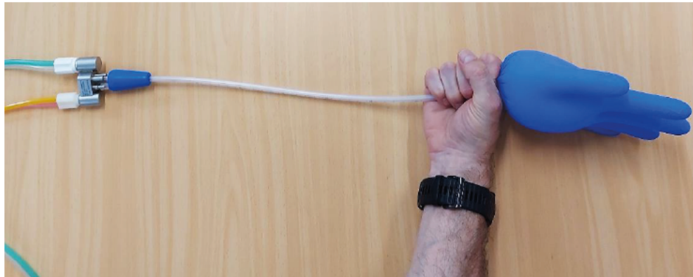
Figure 6: Pressure test. Ventilation is running. Glove inflates.
