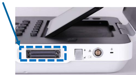
Figure 3. Port on the side for a directly connected transducer
