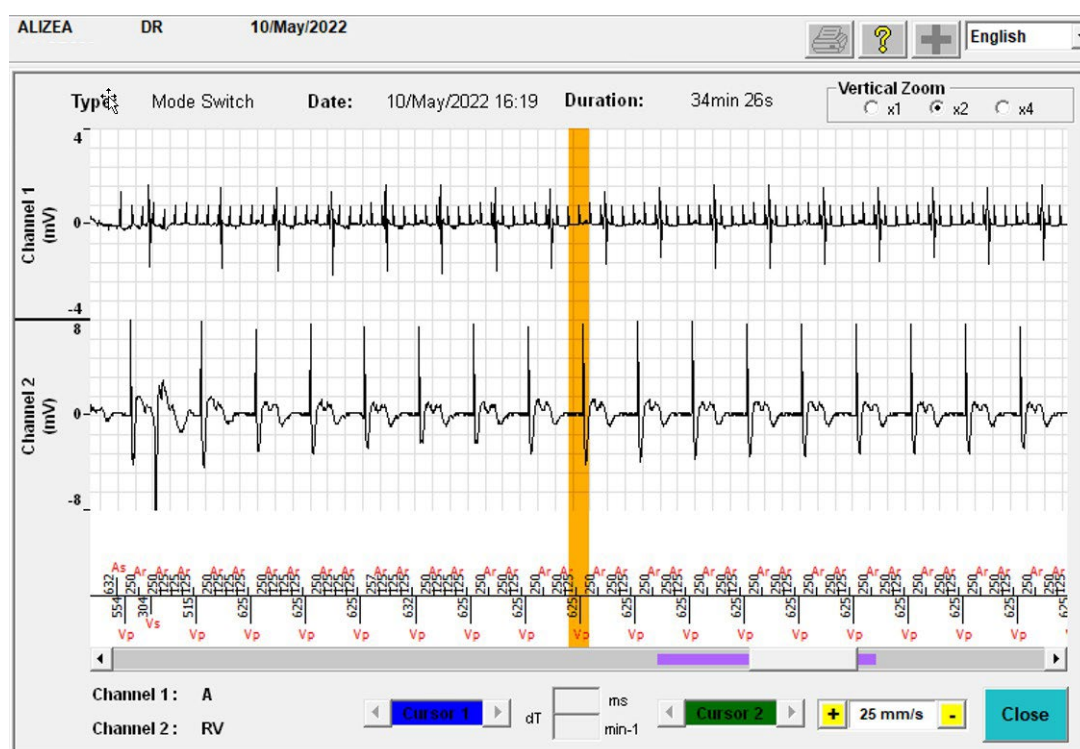
Figure 4: Illustration of “Mode Switch” episode due to MV noise oversensing on a DR pacemaker
