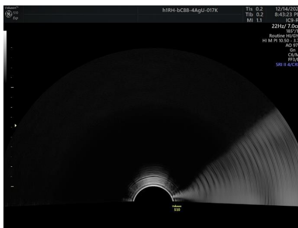
Figure 2. Test image from a normal IC9-RS probe. No artifact visible.
