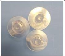
Picture 1 – Incorrect filter connectors with occluding fleece.
