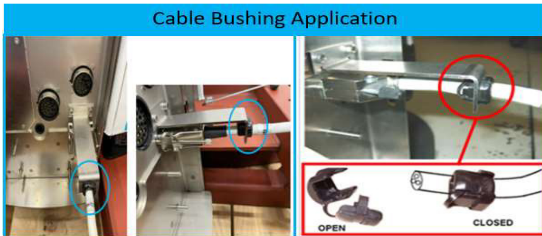
Figure 4b: AD7NT Patient Table with cable tie strain relief
