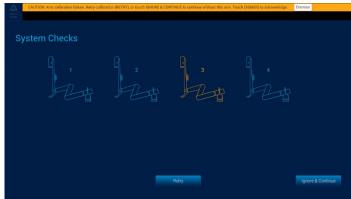
If an arm has failed calibration, <u>do not</u> select the **Retry** or **Ignore & Continue** button. Instead, restart the arm by performing the following steps:
