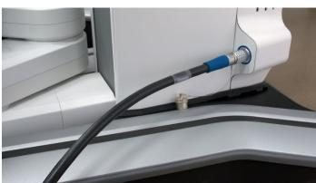
b. Reconnect the arm cart data cable. When the arm completes its startup, the arm cart LEDs will be green and the system will detect the connected arm and display the following message:
