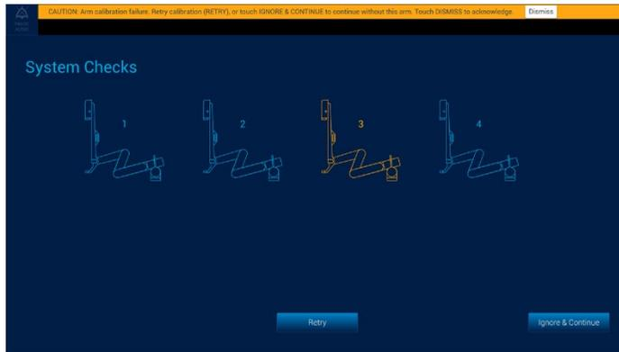
If an arm has failed calibration, do not select the **Retry** or **Ignore & Continue** button. Instead, restart the arm by performing the following steps:
