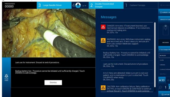
3. If either of the following errors appear in the list of messages, restart the arm according to the instructions in Step 1. If the error appears again, shut down the arm by unplugging the arm cart data cable and remove the arm from service.
