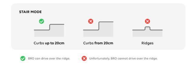
This mode has to be chosen latest before the front of the tracks are over the edge of the step (in drive mode we recommend a minimum of 50 cm of safety distance to switch to stair mode).
