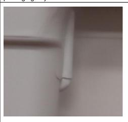
Not conform: Crack in intellipack packaging tray
