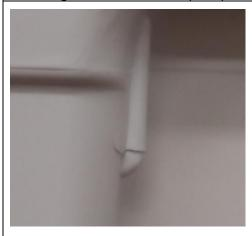
Example for a crack in intellipack packaging tray
