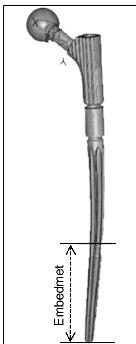
Figure 1: Test setup and marking of embedment
