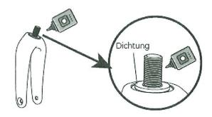
**2.2.5** Reattach the front fork to the frame with the M12 bolt. Tighten the bolt with a torque of 13 Nm. Tool:
