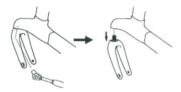
**2.2.4.** Apply glue to the thread only. Please ensure that the gasket remains on the screw for reassembly.
