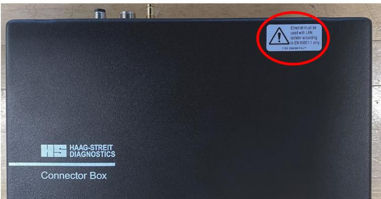
If the warning sticker on the connector box is not in place, it must be applied on the top of the device, above the Ethernet port.
