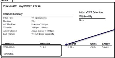
Episode Text example showing *Delivered* reduced shock energy for Rx1; 31.4J when programmed 40J *Energy*.
