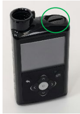
Battery cap on pump
