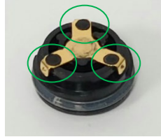
Undamaged battery cap - Continue to use
