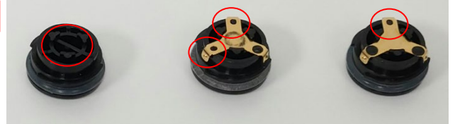
Damaged battery caps - Do not use Metal contact is missing, or fewer than 3 raised
