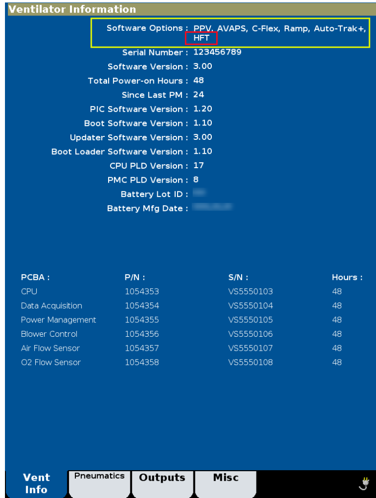
Figure 5: Vent Info tab. Refer to the Software Options list at top of the Vent Info Screen
