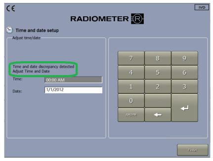
• The operator must then adjust time and date and touch Restart to confirm and restart the analyzer.
