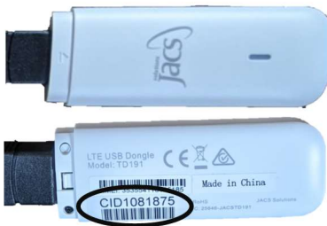
Figure 1. Front/Back images of the 4G LATITUDE MIMIC Cell Adapter, the CID label includes the serial number.
