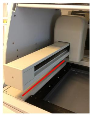
Visually inspect the left plate, area highlighted in red, for signs of unexpected leakage (salt residues and/or liquid). This might indicate leakage from the robotic arm.
