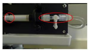
Visually inspect the syringe tray, syringe and stopcock, areas highlighted in red, for signs of unexpected leakage (salt residues and/or liquid).
