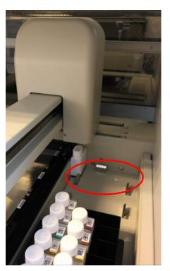
Visually inspect the area around the wash station, area highlighted in red, for signs of unexpected leakage (salt residues and/or liquid). This might indicate leakage from the z-head or too high pump pressure.
