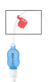
Example of a melted valve opener after the autoclaving procedure at temperatures of 134°C:
