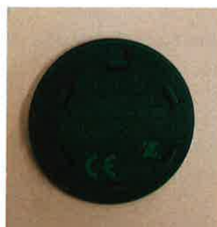
Picture 2: Incorrect color coding (Green) for Item 01.04239.730
