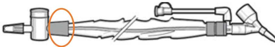
Figure 2: Location where the potential occlusion was identified. The blockage is not visible to the user.
