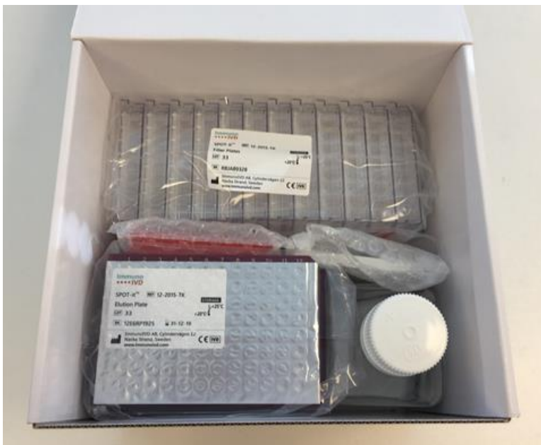
Fig 2. Box insert of kit Box 2 containing additional kit components: elution plates, filter plates, rinse solution, frames, and seals.
