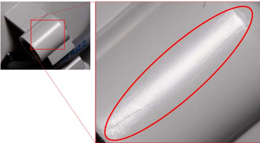
Figure 2. Example of knit line from manufacturing process (Acceptable)
