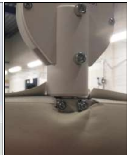
Figure 2: Move the padded cover of the yoke out of the way to expose the screws.
