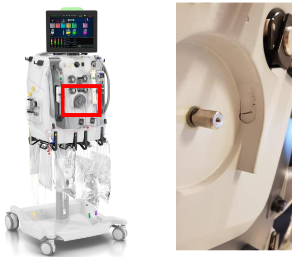
Figure 1: Pictures of PrisMax device and cracks in the blood pump raceway
