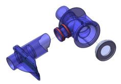
We have detected premature hardening of the silicone membrane, depending on the product used, during the immersion disinfection phase. The rigidity of this membrane may have a negative impact on the quality of ventilation when the PEEP (Positive End-Expiratory Pressure) is set at 0 cmH20 or is virtually zero. It may cause a leak at the expiratory valve, which does not allow the patient to be correctly ventilated.
