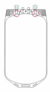
The observed location of the leakage is in the area of the twist-off port weld in platelet storage bags.
