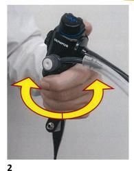
With attached suction tube: While using rotation movement <u>avoid pulling the</u> <u>attached tubing</u>. Assure to have <u>sufficient</u> <u>tube length</u> available in order to avoid pulling forces to the suction valve's main
