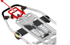
S4453\_FP\_1354100\_Operation09\_Rev01 Let go of the release handle and lift or lower the backrest slightly until it 4 engages
