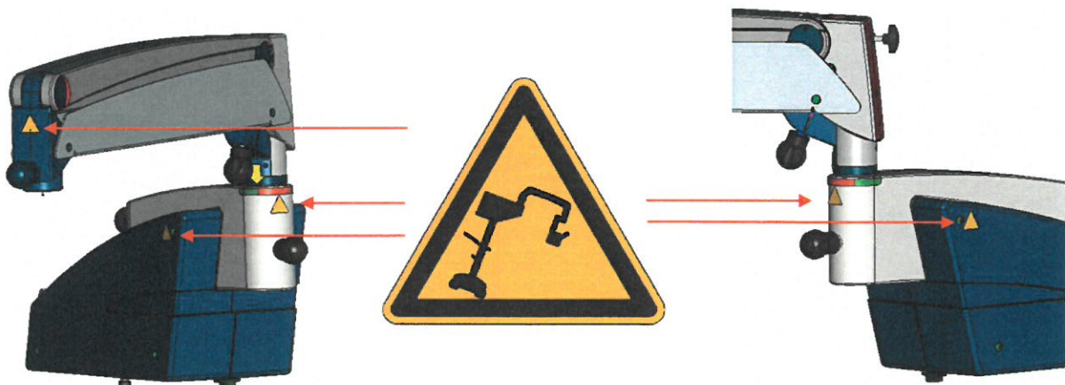
Figure D: Position of new Warning Label
