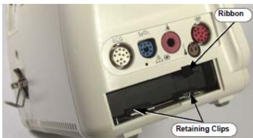
6. Orient the replacement battery so that the contacts and ribbon are on the right.
