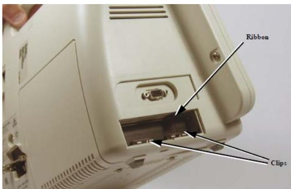
6. Orient the replacement battery so that the contacts and ribbon are on the right.
