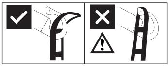
The sling bar hook design prevents sling to be inadvertently detached when mounted correct.
