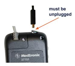
Recharger must be unplugged. Do not reset the recharger while it is plugged into the AC power supply. 2 REMOVE ACCESS COVER
