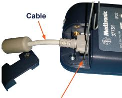
Press and hold reset button for 2 seconds. Replace access cover and tighten the screw.
